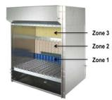
AXIe also includes an optional customizable backplane area known as Zone 3. Essential it is an empty space where a custom backplane may be inserted, or signals can be routed. Since standard AXIe-1 modules don't access Zone 3, they may be inserted into a chassis that does so, without conflict. These features together make AXIe an attractive platform for system integrators.
