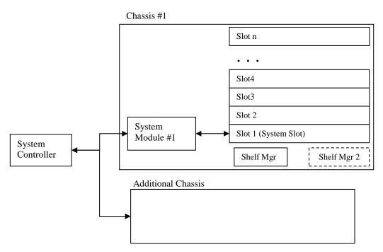
Figure 1 Hardware Components of an AXIe System
